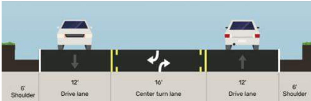
Figure 13. Existing Typical Cross Section from Kerber Drive to Hunter Creek Road (Facing South) – no center turn lane in some areas
