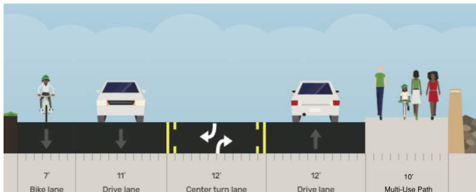
Figure 12. Recommended Typical Cross Section from Jerry's Flat Road to south of Harbor Way (Facing South)
